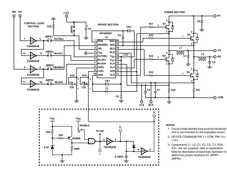
FIGURE 12. HIP4080 EVALUATION PC BOARD SCHEMATIC
