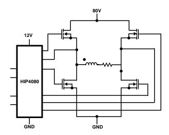
FIGURE 1. HIP4080 SIMPLIFIED APPLICATION DIAGRAM
